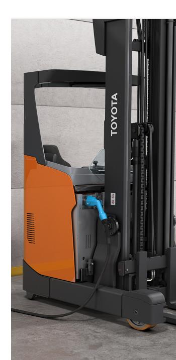
Switching to lithium-ion can be the catalyst for a warehouse redesign that enables a new degree of productivity. Unlike leadacid batteries, lithium-ion does not require dedicated charging rooms; charging points can be located anywhere, including within work areas. Therefore, more of your facility can be freed up for core revenue-generating activities, and you can rethink your layout to optimise flows and maximise efficiency in your operations.
