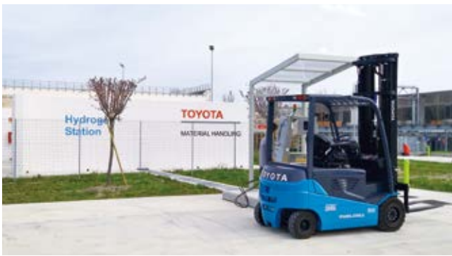
Hydrogen station and a fuel cell lift truck (LTE)
